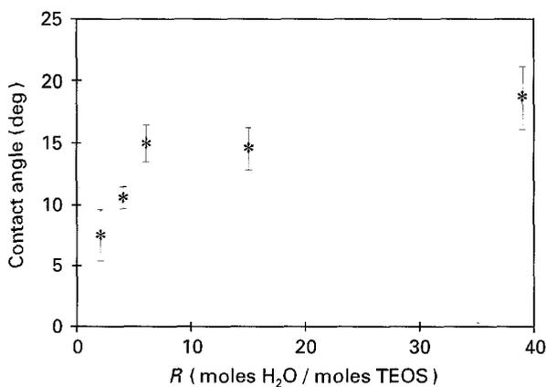
Figure 2 Average contact angle of film-forming solutions on etched silicon as a function of  $R$  (number of moles of water/number of moles of TEOS).
