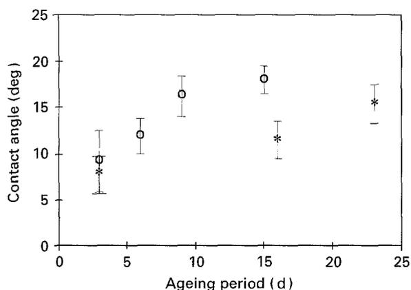
Figure 3 Average contact angle of two film-forming solutions on etched silicon as a function of their ageing time: (○)  $R = 2$  pH = 0; (\*)  $R = 2$  pH = 2.5.
