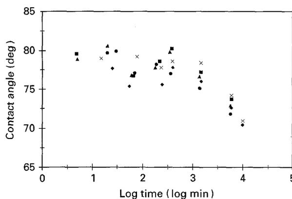
Figure 1 Average contact angle of water on etched silicon wafers as a function of the logarithm of the time of exposure to the ambient.
